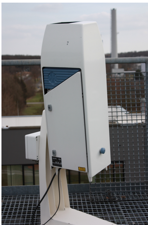
Figure 1.3: Vaisala CT25k ceilometer on the rooftop of the Jülich supersite.
