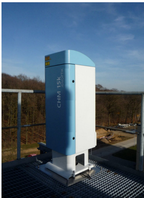
Figure 1.4: Jenoptik CHM 15k NIMBUS ceilometer on the rooftop of the Jülich supersite.
