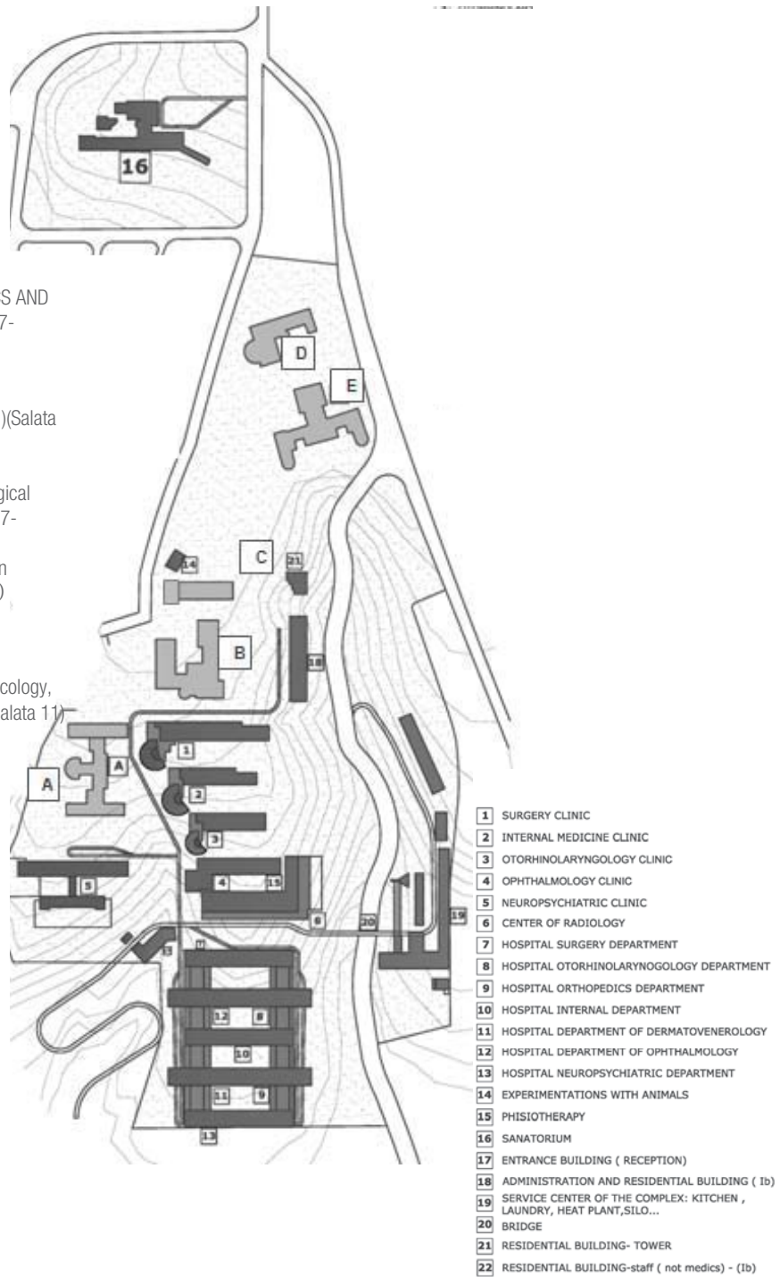
FIG C9 Plan of the whole complex, with the main paths of the complex and access to the buildings. A,B,C and D are the existing building of the clinics and the School of Medicine (F.Gabric 1917-1939) behind the lot of the competition
