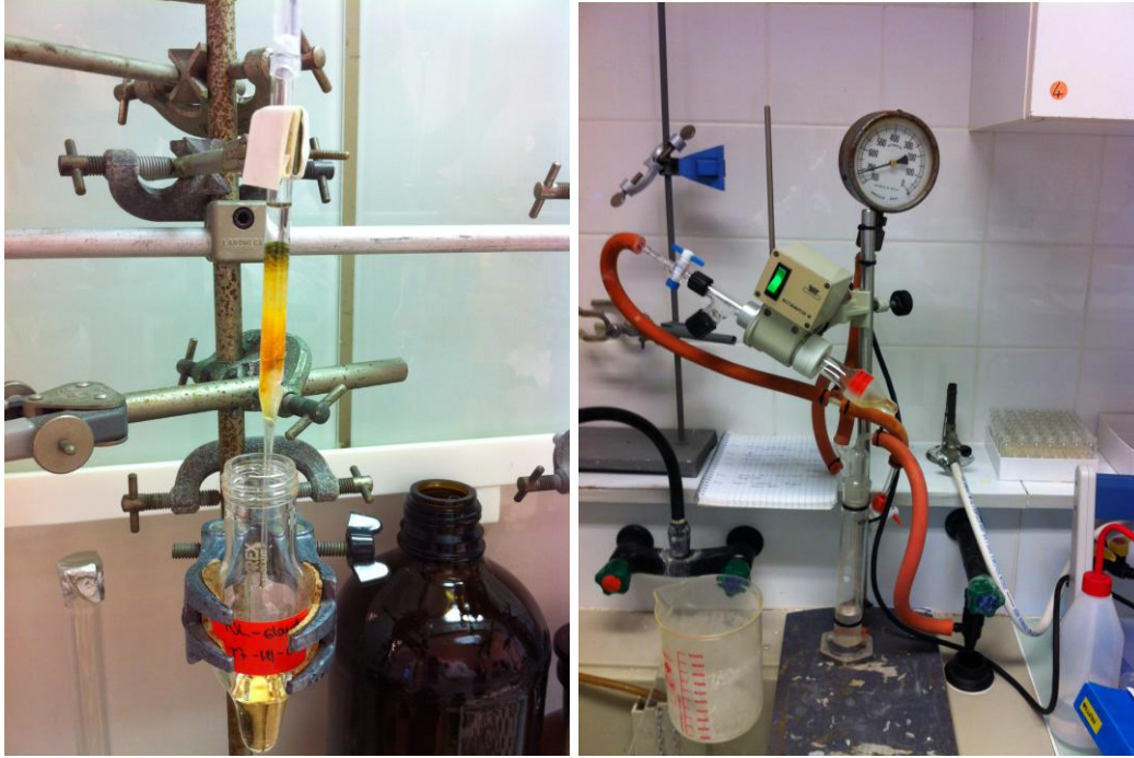
Figure 18. Fatty acid separation (Neutral and Polar lipid) through a silica microcolumn (left) and evaporation of lipid extraction to dryness under nitrogen conditions (right).
