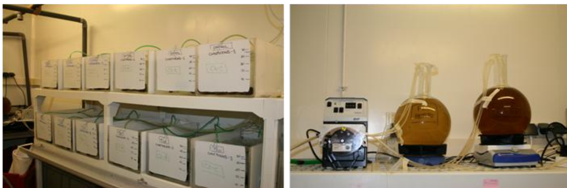
Figure 16. Mussel exposure carried out under controlled laboratory conditions. Mussels tanks (left) and food+toxicant supplied during the exposure through a peristaltic pump (right).
