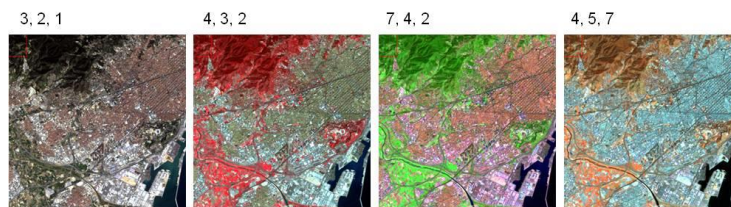
Fig. 4.17: Some of the most common band combinations, for Landsat TM multispectral imagery: Natural Colour; Colour Infra-red (CIR); Pseudo-Natural Colour; and Infrared based combination (Source: by Authors)
