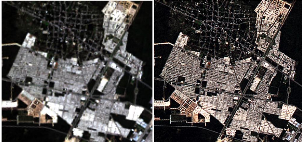
Fig. 4.19: Pan-Sharpening transformation result (Right side) for a multispectral Landsat image, at 30m resolution (left side), combined with a Landsat 15m panchromatic image (Source: By Authors)
