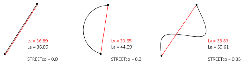
Fig. 5.13: Sample of the Street Complexity Index ( STREET_{co} ), calculated for three different linear objects (Source: By Authors)
