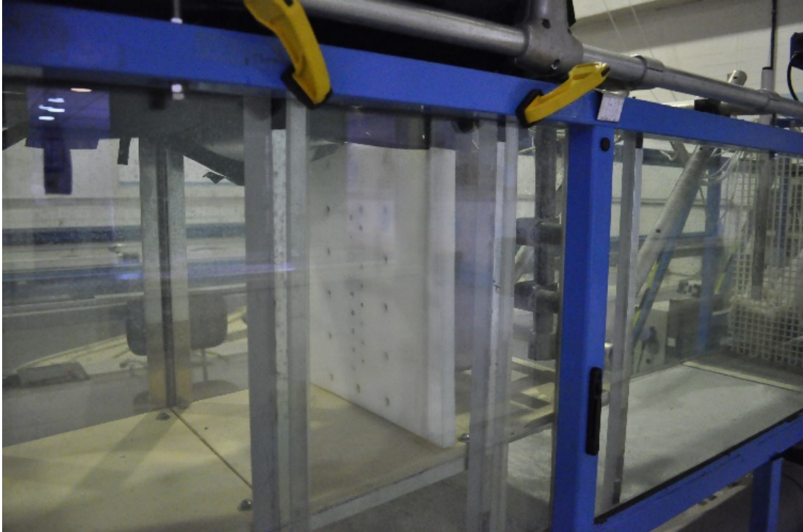
Figure 3.3: Vertical wall mounted in the CIEMito wave flume
