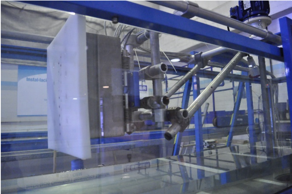
Figure 2.2: Reticular structure that constrains the load cells
