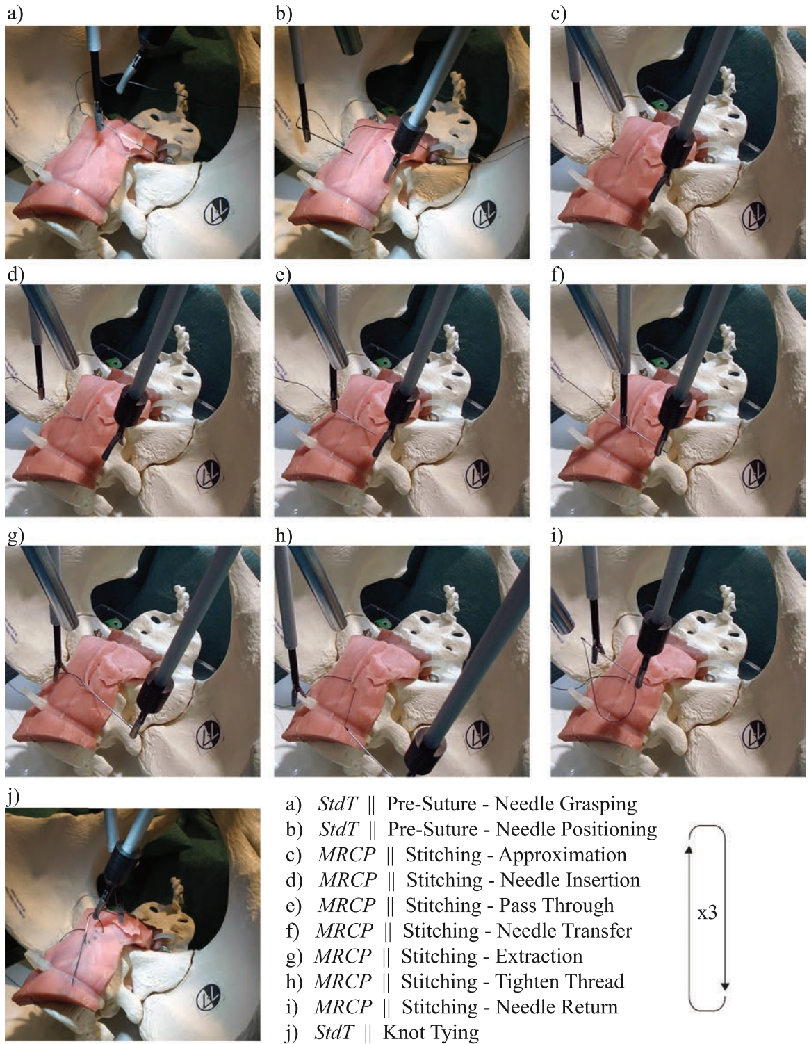
Figure 5.37: Complete process of a suture with three stitches using the combined approximation: StdT and MRCP
