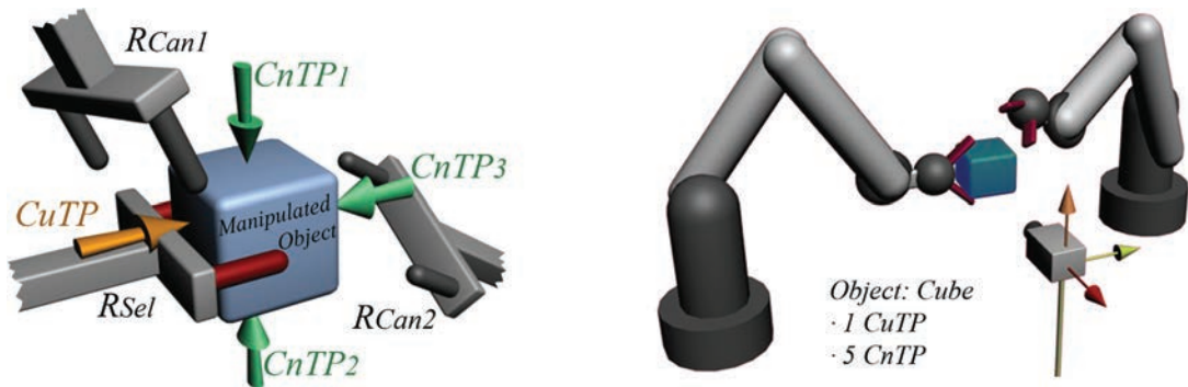
Figure 4.12: Illustrative example of telemanipulation of a cube with 6 pre-defined grasping positions
