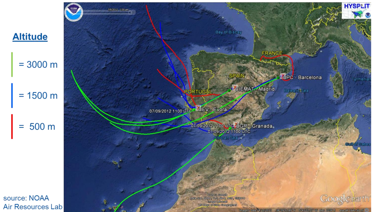
Figure 2.3 Two-day backward trajectory analysis from the NOAA HYSPLIT model, with endpoints of the four lidar stations on 9 July 2012. The analysis is performed arriving at three heights; 500-m, 1500-m, and 3000-m.
