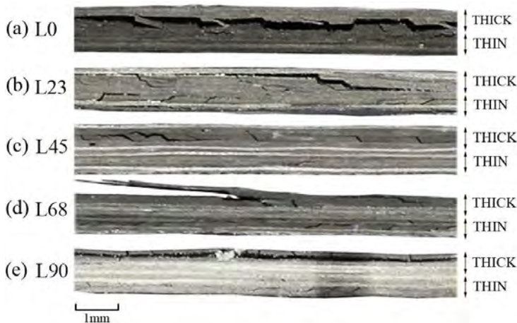
Fig. 3.3: Crack growth for each lay-up just before ultimate failure [43].
