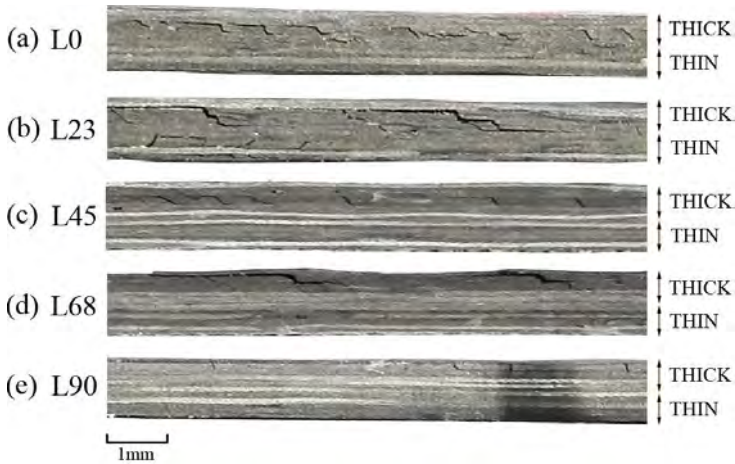
Fig. 3.1: Damage occurrence under an applied strain of 1.25% [55].
