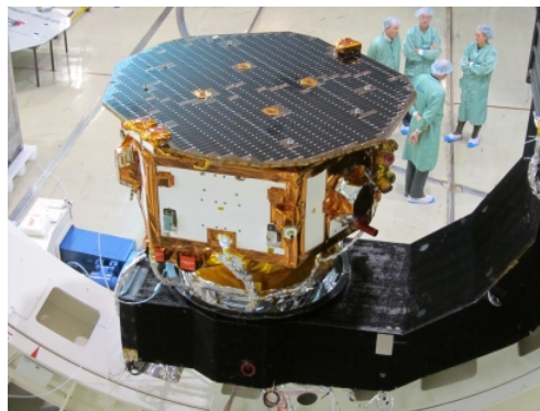
Figure 1.23: LISA Pathfinder during the On-Station Thermal Test (OSTT) in Autumn 2011. Credits: Airbus Defence and Space UK.
