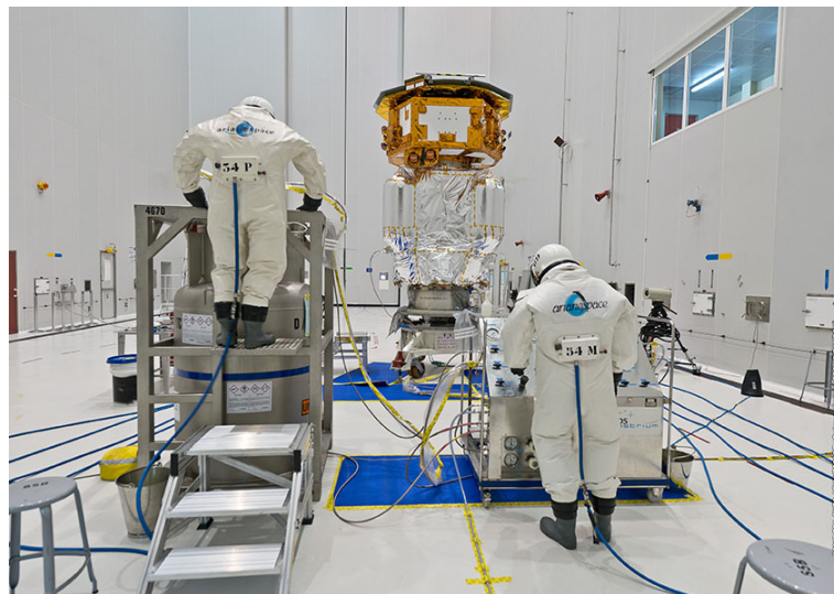
Figure 7.1: LISA Pathfinder in the S5B building at the Centre Spatial Guyanais in Kourou, French Guiana, while filling the propulsion module with propellant (November 2015). Credits: ESA-CNES-Arianespace / Optique Vidéo du CSG - P. Baudon.
