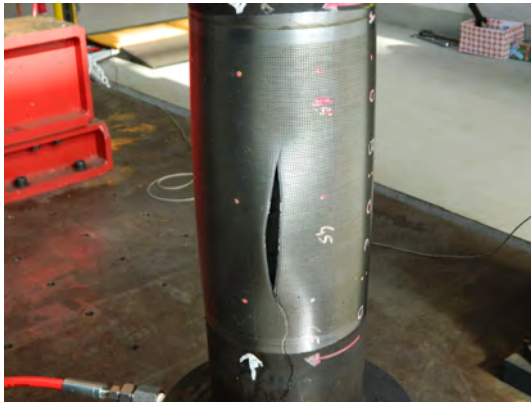
Figure 3.48: View of the pipe burst as recorded by the experiment for the SPEC1 test
