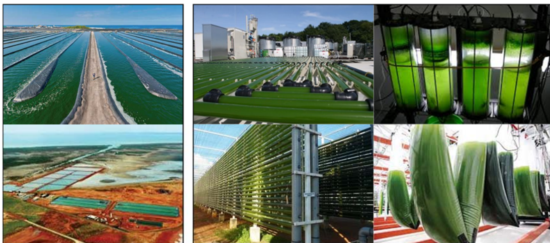
Figure 2. Microalgae production technologies at large scale; open ponds (a) and closed photobioreactors (b).
