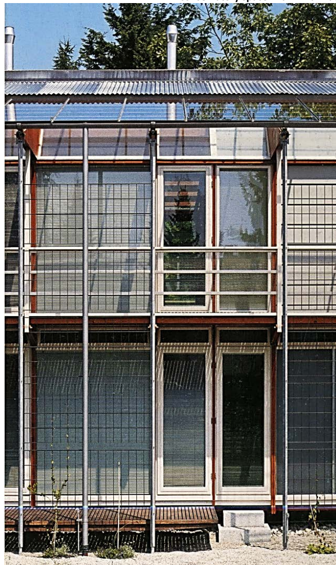
Figure 38: Two-family House, Pullach, South face with translucent thermal insulation elements, Ground-floor
