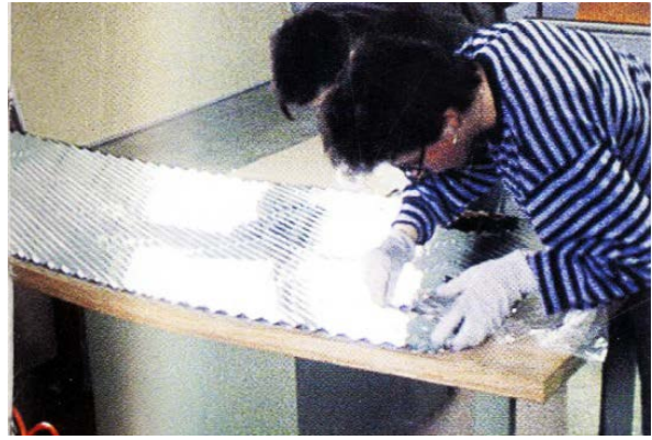
Insertion of grid elements between layers of double glazing
