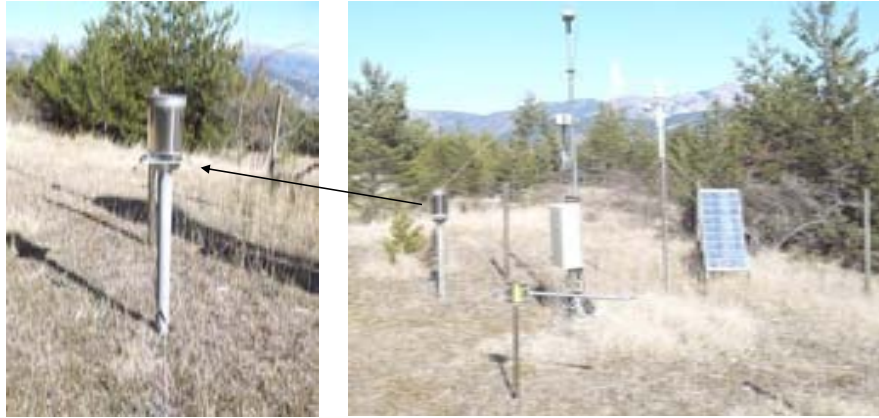
Figure 6.3: Rain gauge in Vallcebre catchments.
