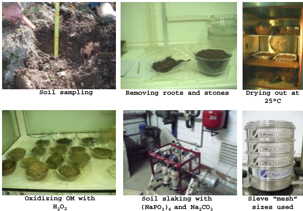
Figure 6.8: Main steps for texture determination.
