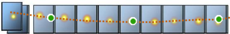
FIGURE 4.5: A scene record parametrizes the object transit providing three predicted knots over the trajectory of the transit over the focal plane in the SRS - from SM (left) to AF9 CCD
