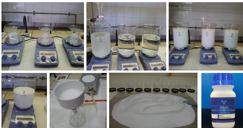
Figure 1. Synthesis of PSm performed at the laboratory through the organic solvent extraction/evaporation methodology.
