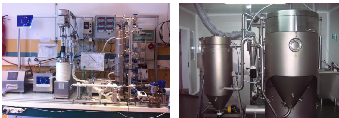
Figure 15. Equipment employed for the micronisation of PSm: (A) Supercritical Fluids; (B) Closed cycle Mobile Minor TM .
