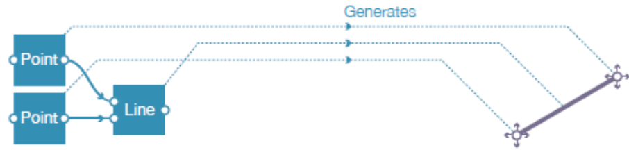
Figure 34: The relationship between a DAG and the geometry it generates. In the DAG the line is a child of the two points, accordingly, the line's geometry depends entirely on the location of the points. Moving the geometry of either point would also move the line.
