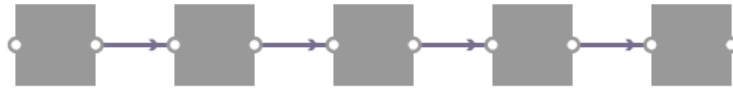
Figure 17: A directed acyclic graph comprised of a single path, which gives it a cyclomatic complexity of one.
