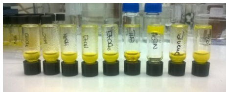
Figure 4. Picture of the tube inversion tests with gelator 1b previously dissolved in DMSO.
