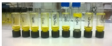
Figure 15. Picture of the tube inversion tests with gelator 1b previously dissolved in DMSO.
