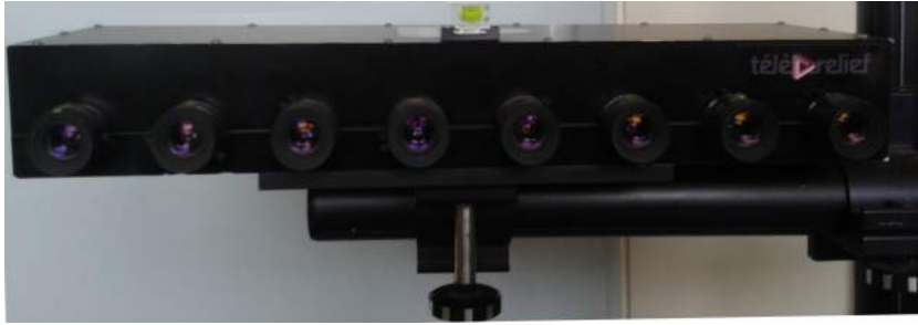
Figure 4.3: The Octo-cam, multi-view camera prototype.
