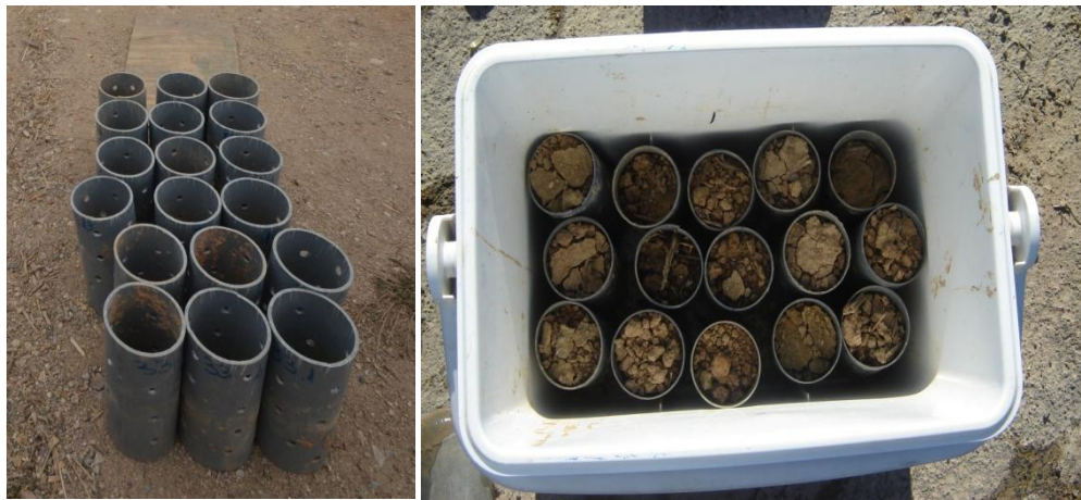
Fig. 3.3.5 The PVC tubes used to take undisturbed soil cores from the super-intensive olive tree orchard
