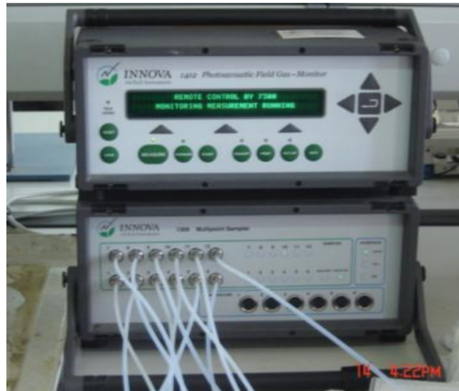
Fig. 3.2.1 Photoacoustic analyser (Innova 1412 Photoacoustic Multigas Monitor)
