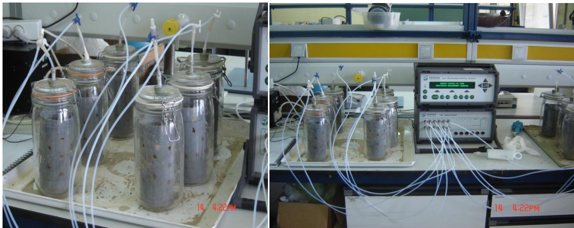
Fig. 3.3.7 The glass jars (1.5 L) with air-tight glass lids, containing the undisturbed soil cores collected in the PVC cylinders (a) and the connection between the glass jars and the photoacoustic analyser (Innova 1412 Photoacoustic Multigas Monitor) via Teflon ® tubing (b)
