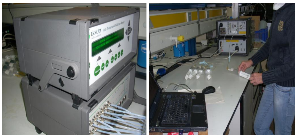
Fig. 3.3.4 Analysing the samples of N_2O , CO_2 , CH_4 and N_2O+N_2 using the photoacoustic technique
