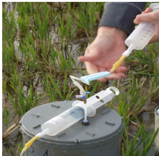
Fig. 3.2.3 Taking samples of air inside the closed chamber
