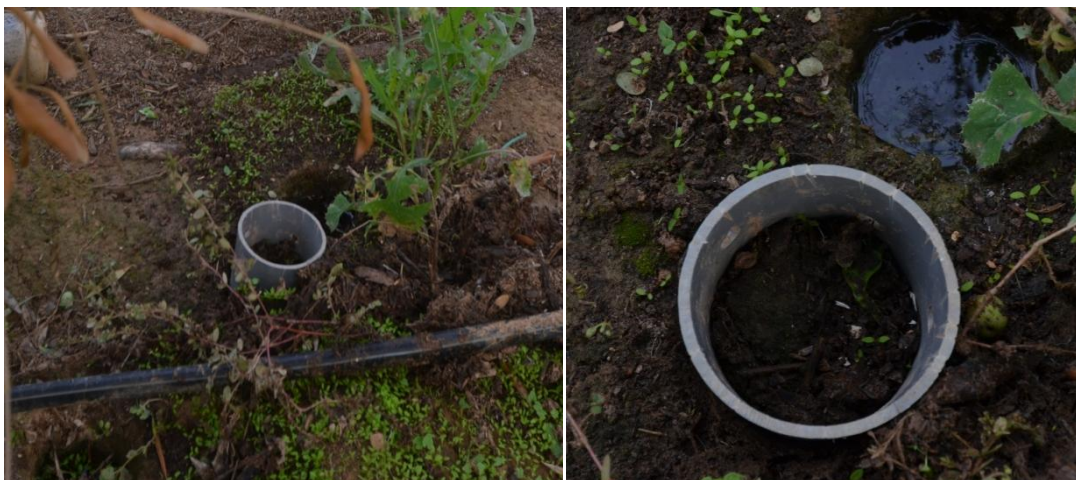
Fig. 3.3.6 The undisturbed soil cores were taken from the wet bulb
