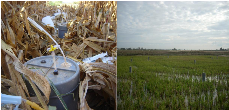
Fig. 3.2.2 Views of the gas sampling chambers used on maize (a) and on rice (b)
