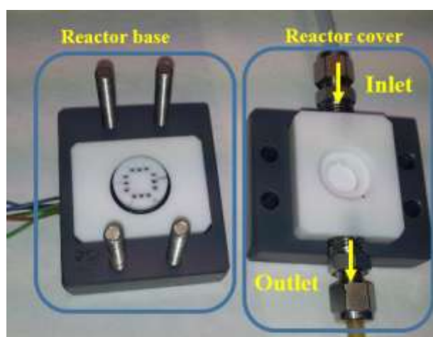
Figure III.5. AACVD cold wall reactor adapted for MEMS sensor packaging.
