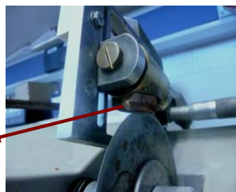
Figure 2.2 b) Diamond saw for cutting the sample
