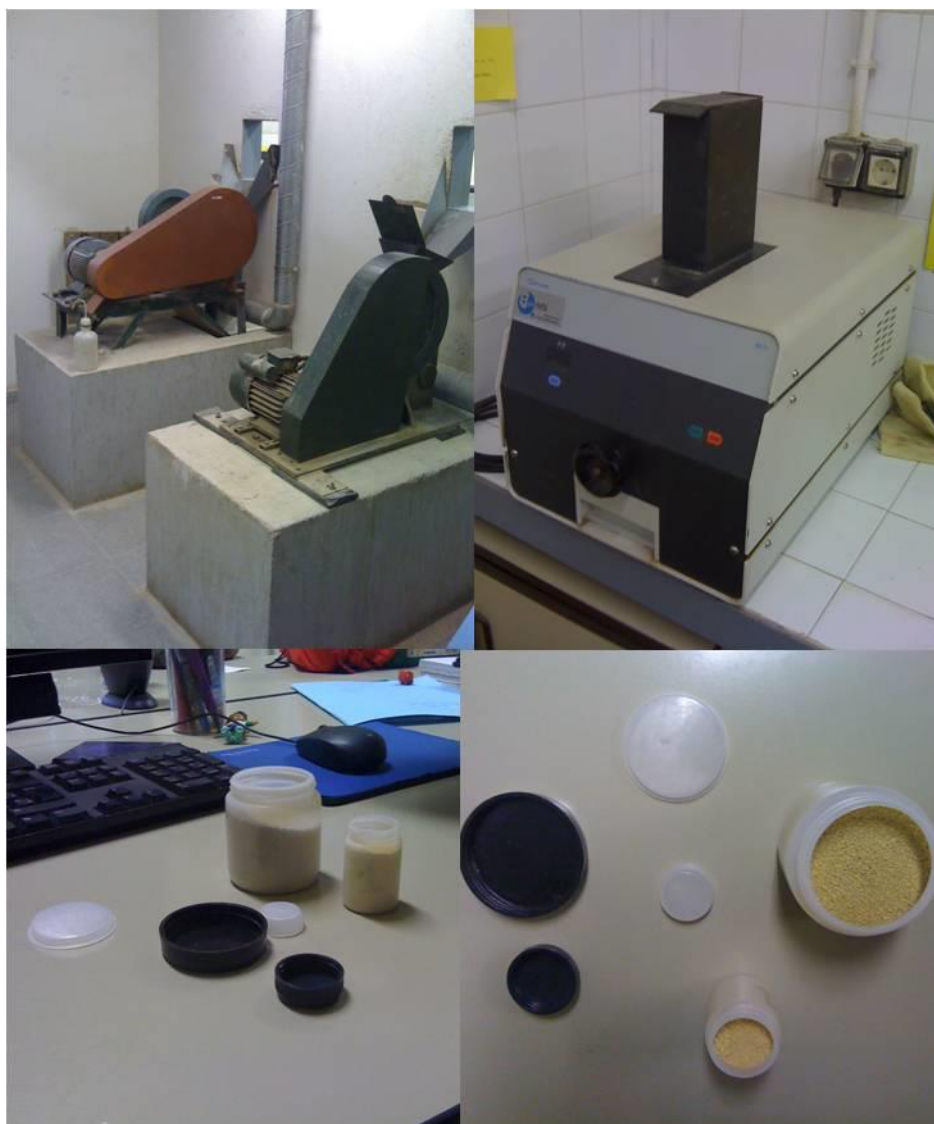
Figure 0-92: Top-left: Jaw crusher used to reduce samples to an appropriate grain size to be introduced in the disc mill (top-right) to obtain the final grain size (250-1000 \mu\text{m} ). Samples were stored in plastic (bottom) pots to be treated later.
