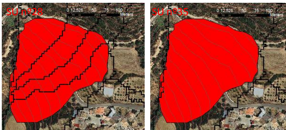
Figure 5-17: Left: Mapped landslide (red) cut by SUs when using too small mapping units (SU no. 28). Right: SUs of higher areas have been delineated to fit better with the mapped failures (SU no. 35).
