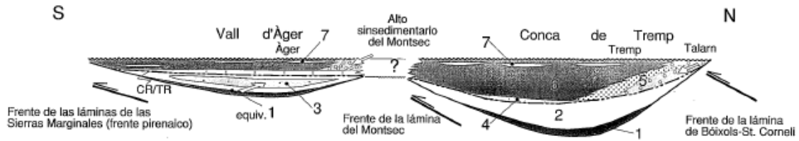
Figure 2-4: Simplified cross section of the Tresp Basin (from Rosell et al., 2001). No vertical scale. Horizontal scale: 50 km. 1 ) Grey Garumnian. 2 and 3 ) Lower Red Garumnian. There are expansive red clays at the bottom. The other part is affected by pedogenic processes with small channels. 4 ) Vallcebre Limestones. 5 , 6 and 7 ) Upper Red Garumnian: Dejection cones with conglomerates and sandstones (5), marly paleosoils and lacustrine limestones (6) and evaporites (7).
