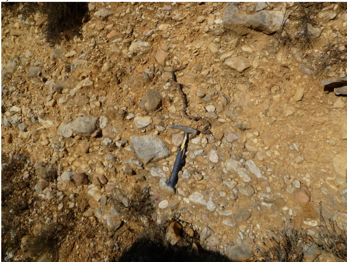
Figure 3-7: Coarse colluvium. Clast supported with clayey, silty and sandy matrix from Garumnian (Photo: Guillem Domènech).
