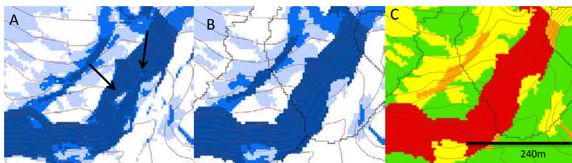
Figure 5-21: A) Reclassified susceptibility map obtained from SINMAP; B) Susceptibility map after pixel clustering using SU no. 40; C) Hazard map obtained after the application of the MF matrix (Table 5-12).
