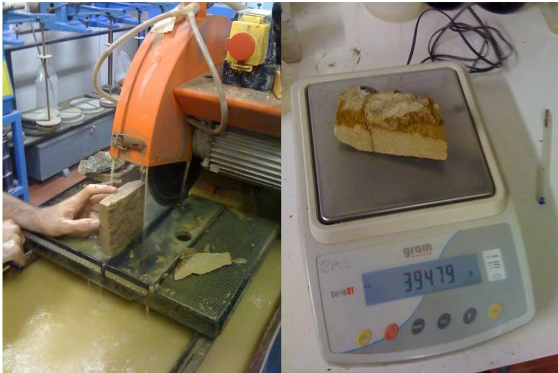
Figure 0-91: First millimetres of samples were sawn to eliminate rusty or weathered surfaces noting the thickness of soil removed.
