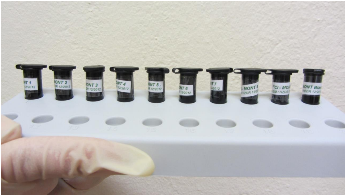
Figure 0-93: AgCl obtained from the second precipitation and ready to be measured by the AMS. It must be kept from light due to its photosensitivity.
