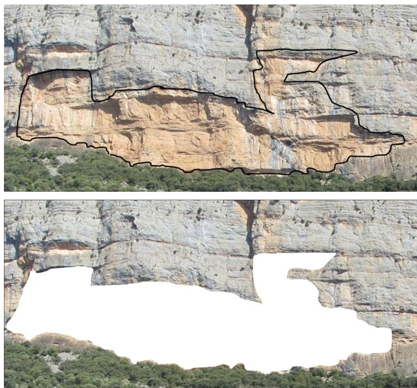
Figure 7-9: Delimitation of the rockfall scars area based on its colour and the depression of the topographic surface (Z1) (Top). White mask overlaying the area affected by rockfall scars (Z1) (Bottom).
