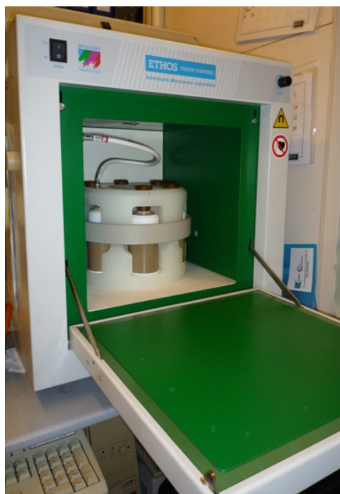
Figure 2.1-2. Microwave equipment (Milestone Ethos Touch control).
