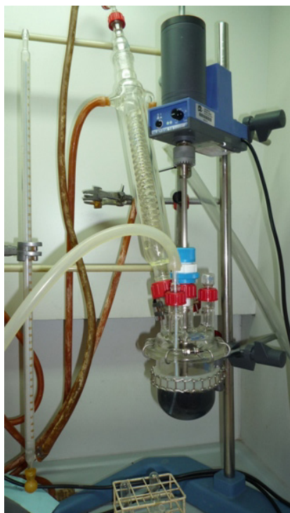
Figure 2.3-1. Assembly used in the catalytic tests for the hydrogenation of styrene oxide.
