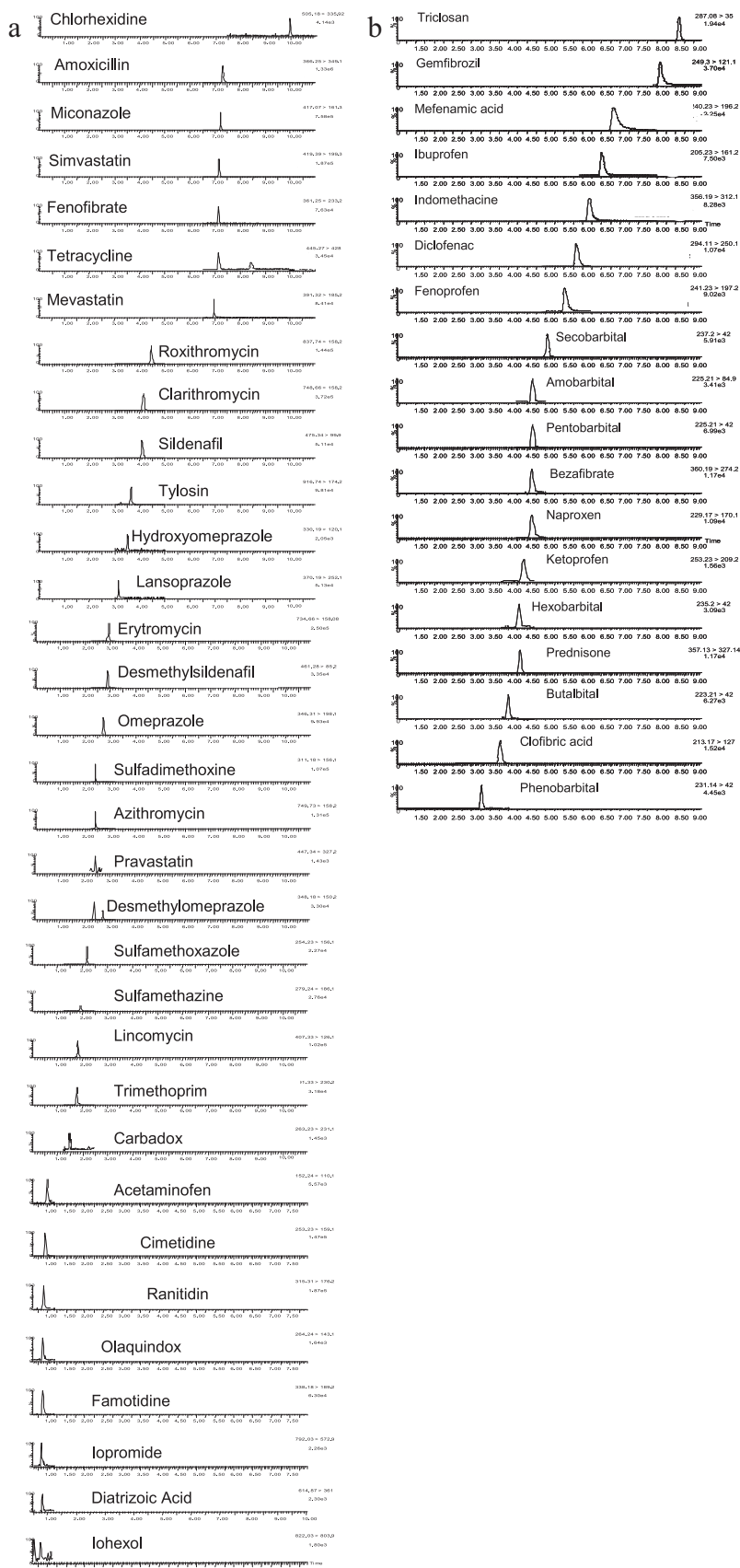
Fig. 1. UPLC-MS/MS extracted ion chromatogram of target pharmaceuticals in ESI positive (A) and negative (B) modes.
