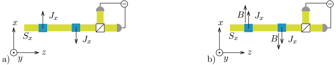
Figure 6.2: Sketch of the experimental setup applied in [79] to generate bipartite entanglement. a) Entangling pulse. b) Verifying pulse followed by homodyne measurement. A local magnetic field is added (parallel to the spin polarization direction) in order to measure two transverse components of the spin with a single light beam.
