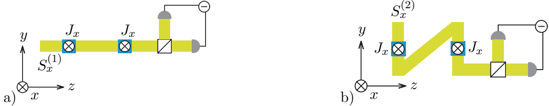
Figure 6.5: Entanglement eraser scheme realized by two pulses of different intensity, \kappa_1^2 \propto N_{\text{ph}}^{(1)} and \kappa_2^2 \propto N_{\text{ph}}^{(2)} . See the text for details.
