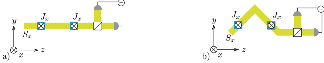
Figure 6.3: The simplest setup for generation and verification of bipartite entanglement between mesoscopic atomic ensembles. a) First light pulse passing through the samples along direction z entangles the samples. b) Second light pulse passing through the samples at angles \pi/4 and -\pi/4 , respectively, allows for verification of entanglement through a variance inequality (see Eq. (6.9)).
