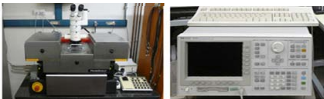
Figure 5.16 Equipment used for the electrical characterization on ambient conditions. (Left) Karl Suss probe station. (Right) HP4155 semiconductor analyzer.
