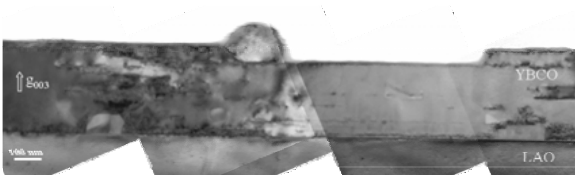
Figure 5-6. Cross-section bright-field TEM composite micrograph viewed along \langle 100 \rangle of the YBCO film taken when the diffraction beam is \mathbf{g} = (003) .
