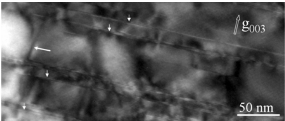
Figure 5-11. High magnification XTEM image taken with a diffraction vector \mathbf{g} = (003) . SF's are signaled by small arrows, while the large arrow signals a threading dislocation.
