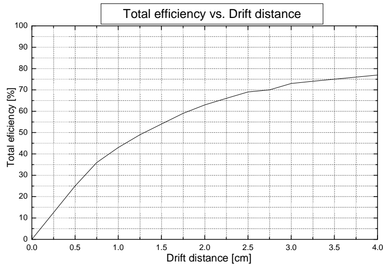
Figure 4. 9 Total efficiency as a function of the drift distance. The x-ray energy is 10keV, the gas mixture is Xe 90% + CO 2 10%. The window is formed by 375 \mu m of carbon and 55 \mu m of kapton; which has a transparency of 81%. In order to have a total efficiency >50%, a drift distance >1.3cm is needed
