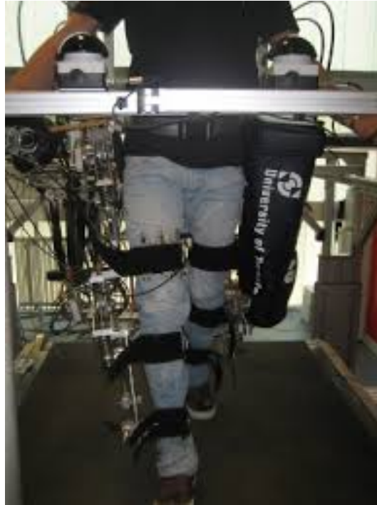
FIGURE 2.7: Illustration of LOPES - Lower Proximity Exoskeleton; The joint actuation in LOPES is adaptive but apparently huge in size because of the actuator model.
