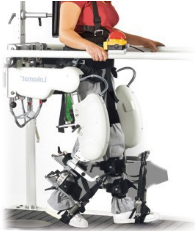
FIGURE 2.6: Illustration of treadmill training device- Lokomat; The BWS is variable depend on the user performance while the speed is always fixed with respect to the treadmill. Lokomat is considered more as a stationary device due to the BWS
