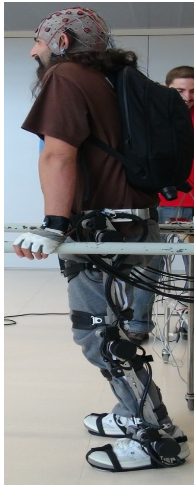
FIGURE 5.22: Experimental setup with an incomplete SCI patient wearing the Exoskeleton and BMI system
