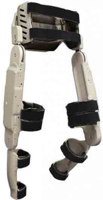
FIGURE 2.12: Illustration of Vanderbilt Exoskeleton; A light weight exoskeleton with hip and knee joints actuated and used in combination with AFO
