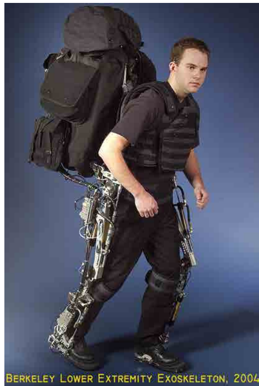
FIGURE 2.11: Illustration of BLEEX- Berkeley Lower Limb Exoskeleton, a performance enhancing exoskeleton
