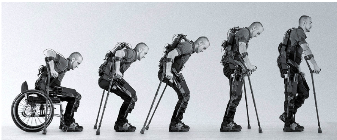
FIGURE 4.1: Rehabilitation tasks in a lower limb therapy- Sit-to-stand; Balance Training and Walking performed using ReWalk exoskeleton [157]
