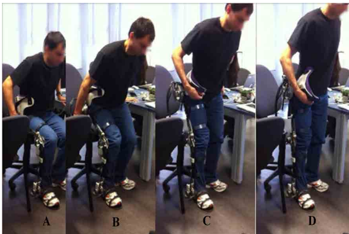
FIGURE 5.2: Sit-to-stand task performed by a healthy subject with the exoskeleton H1
