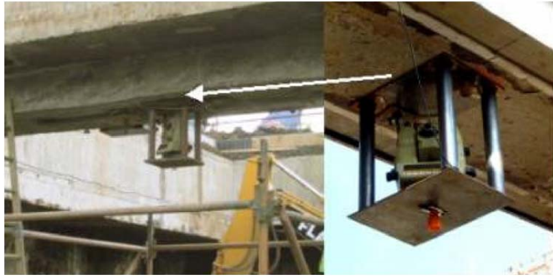
Figure 2.4 The Leica TCA1800 RTS mounted in the TBM shaft (Walker, Hitchcock et al. 2006).
