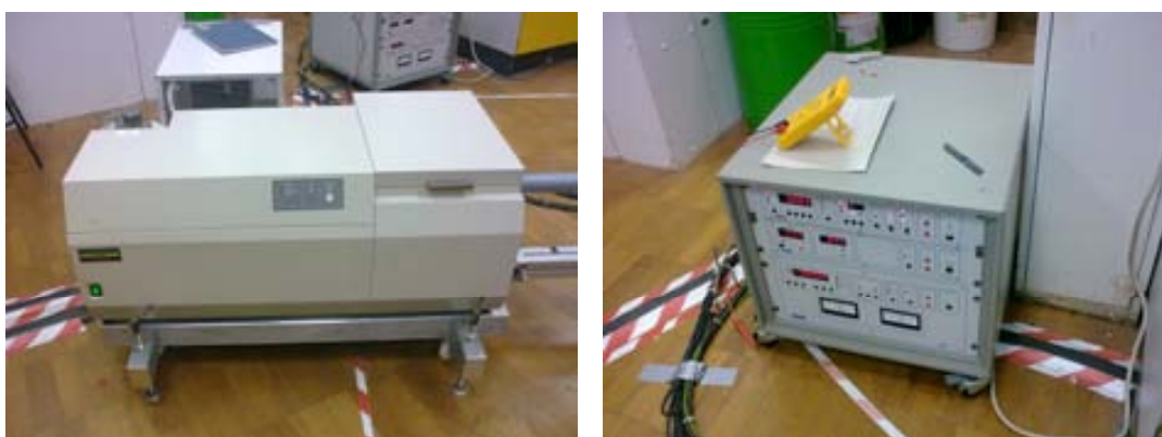
Figure 4-19. JASCO 810 spectropolarimeter (left) and control unit of the 8 T superconducting magnet (right)
