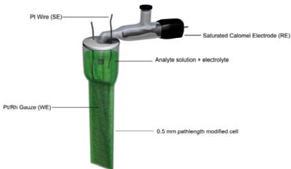
Figure 4-2. Representation of the cell used for spectroelectrochemical characterizations using a transparent Pt/Rh electrode. [13]
