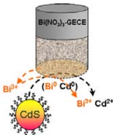
Figure 3.7 Proposed schematic of the electrochemical detection of CdS QDs. Bi 3+ is released from the surface of the electrode and reduced back to Bi 0 together with the Cd 3+ (defects) to Cd 0 . During the stripping process both Bi 3+ and Cd 2+ are released.
