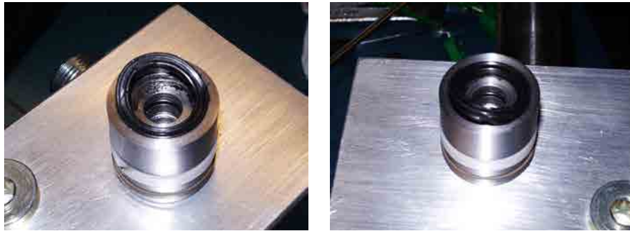
Figure 6.3: O-ring damaged due to excessive compression force on the upper packing of spool valve V_1
