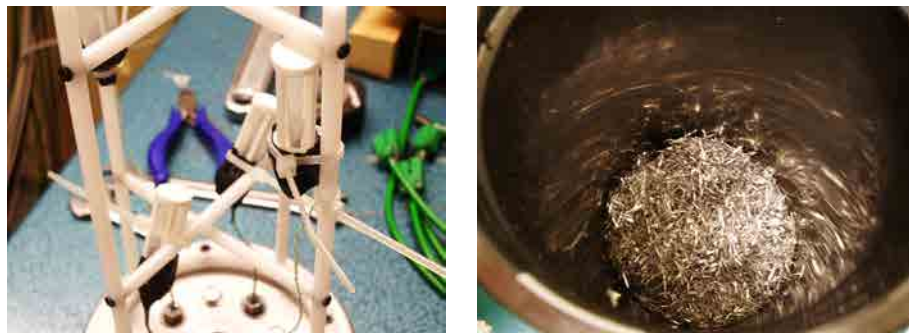
Figure 6.45: (Left view) Plastic encapsulation to prevent from direct contact with the medium. (Right view) Filling material to ensure isothermal condition
