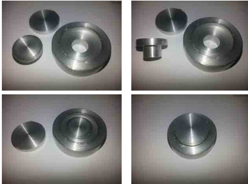
Figure 6.4: View of the tool used to produce polyurethane ring moulded gaskets
