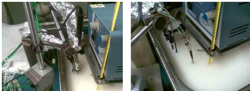
(b) Thermocouples immersed in an oil-bath
