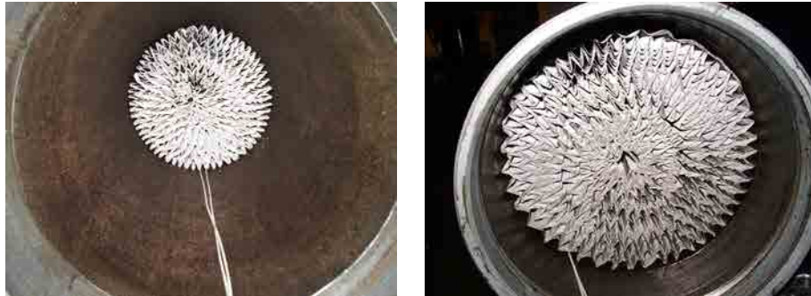
Figure 6.21: Stainless steel wire mesh inside the isothermal tank
