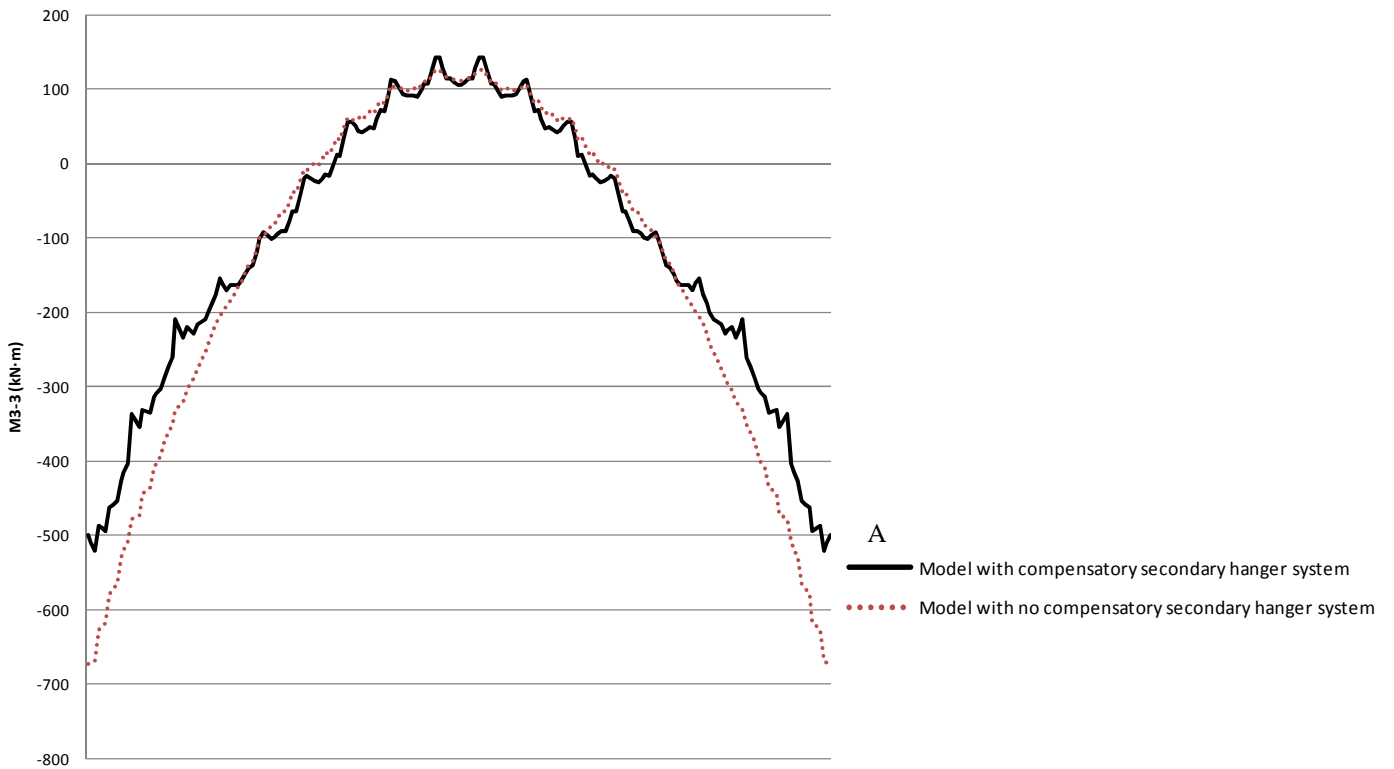
Figure 4-29: Arch in-plane bending moments comparison of models A and B with and without secondary hanger system. The abscissas are the arch length from 0 to L_A
