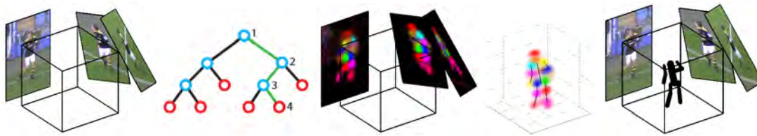
Figure 5.1: Example of a multiview 3D pose estimation approach. In this approach a random forest is first used to classify each pixel in each image as belonging to a part or the background. The results are then back-projected to a 3D volume. Corresponding mirror symmetric parts are found across views by using latent variables. Finally, a part-based model is used to estimate the 3D pose Figure reproduced from (Kazemi et al., 2013).
