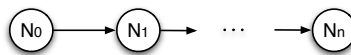
Figure 3.11: Chain topology, where N_0 is sending traffic to N_n , through relays N_i, 0 < i < n .
