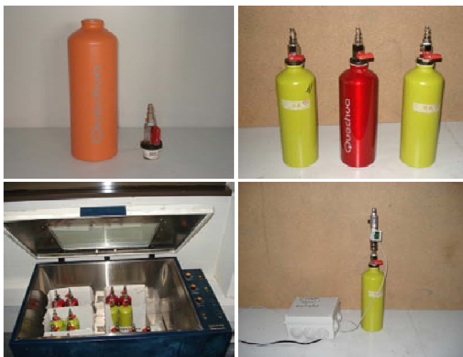
Figure 3.6: Reactors used for anaerobic bioremediation treatments.
