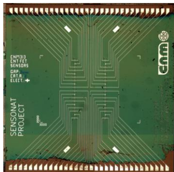
Figure 8.13. Photograph of a sensors chip platform after the CNT-FET structures have been passivated and the PMMA layer has been removed from the pads. The chip is 5 x 5 mm 2 .
