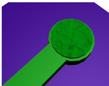
Figure 9.1: Schematic of an electrode and its corresponding stripe. The electrode has been drawn rougher to exemplify the importance of its surface.
