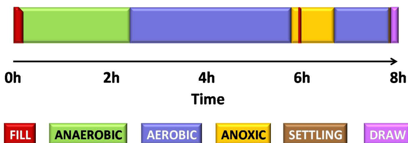
Figure 6.1. 8-h cycle applied in the SBRs for nutrient removal purposes.
