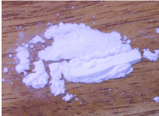
Figure 7. Microencapsulated PCM commercialized by BASF.
