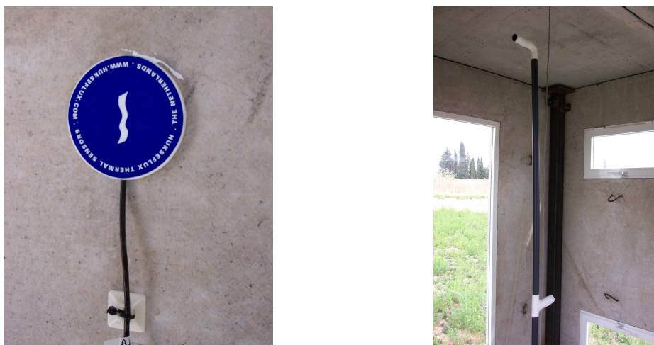
Figure 59. Instrumentation: heat flux sensor (left) and temperature sensor in the middle of the cubicles (right).
