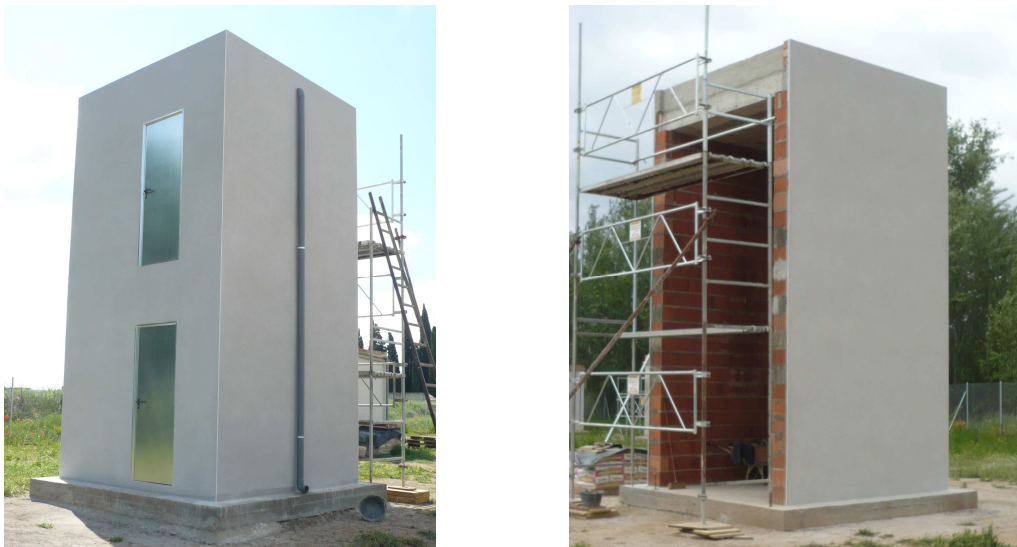
Figure 147. Double height cubicles with an interchangeable nogging for experimentation with ventilated facades with PCM.
