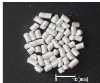
Figure 15. Granulated PCM used by Takeda et al. [221].
