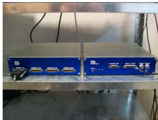
Figure 6. Recording system. Pre-amplifier (left) and analog-to-digital converter (right) allowed to electrophysiological recordings of single units and field potentials.
