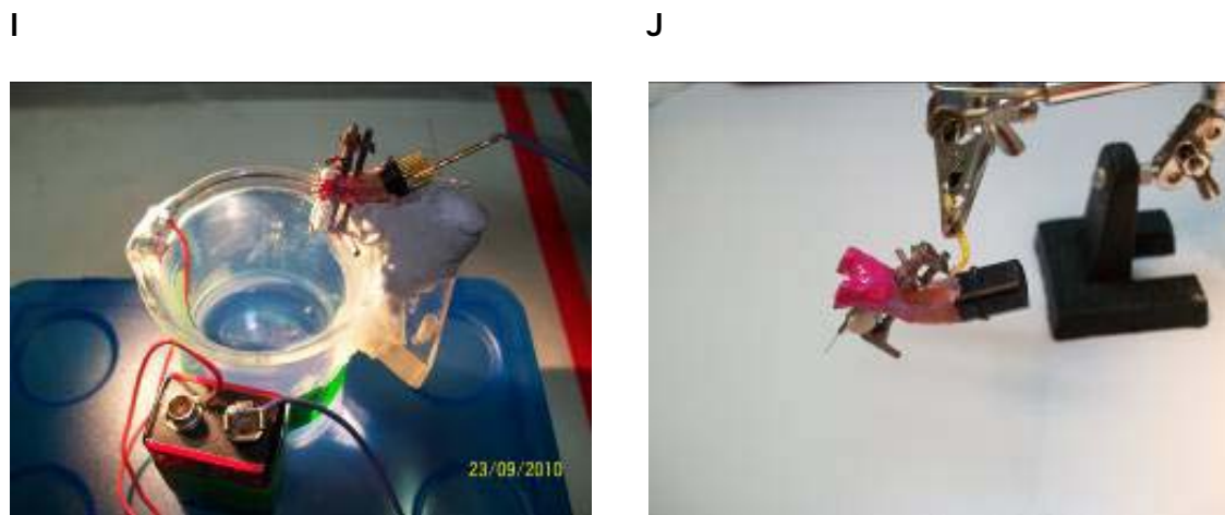
Figure 1. Tetrodes and microdrive making. A,B. Each tetrode consisted of four strands twisted by means of a magnet. C,D. Each tetrode was placed in the cannula of the microdrive. Each tip was burnt in order to remove the isolation and improve connectivity when the electrodes were attached to each cable. E-H. Silver was placed in each cable tip in order to further improve connectivity with each electrode. I. 9 V current was applied to each microdrive channel in order to test for possible shorts. J. Cable tips were covered with nail polish in order to isolate and protect them.
