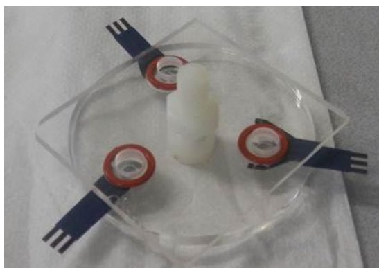
Figure C3: Picture of an example of electrochemical cell with three electrodes right after being assembled, before casting the 200 \mu\text{L} of cell suspension in the well. In red, the rubber rings used to press the anodized aluminum oxide membrane (AAO) on the screen printed electrode (SPCE) can be seen through the transparent methacrylate pieces of the set up.
