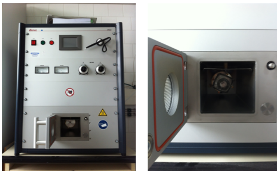
Figure 2.2: Photograph of the RF plasma activation reactor. The sample is loaded in the compartment displayed in the right.
