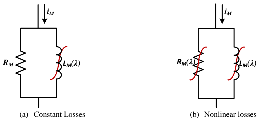
Figure 5.10. Transformer's core representation
