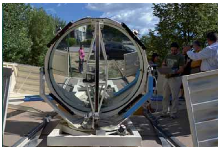
Figure 2.6: Photo of the telescope (parabolic solid-glass mirror of 1.8 m diameter) used by the Barcelona IFAE-UAB team to build their Raman lidar.
