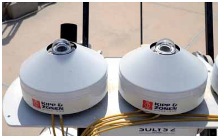
Figure 4.10: Kipp & Zonen CMP11 pyranometers used at the solar radiation monitoring station installed at the QEERI facility. Note the shadow covering the sensor of the left pyranometer, in order to measure DHI.
