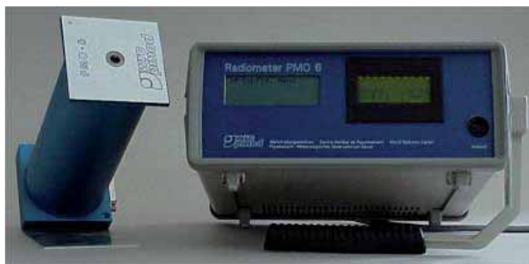
Figure 1.9: Absolute cavity radiometer from PMOD/WRC.
