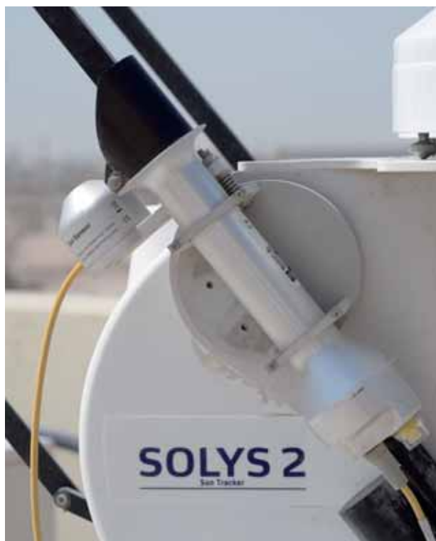
Figure 4.9: Kipp & Zonen CHP1 pyrheliometer used at the solar radiation monitoring station installed at the QEERI facility.
