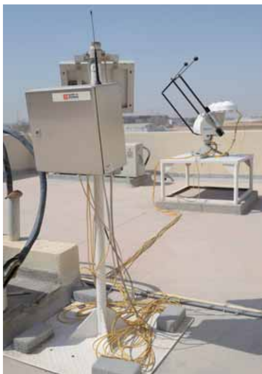
Figure 4.11: Data logger in its enclosure, for the communication of the solar radiation measurements from the monitoring station installed at the QEERI facility.
