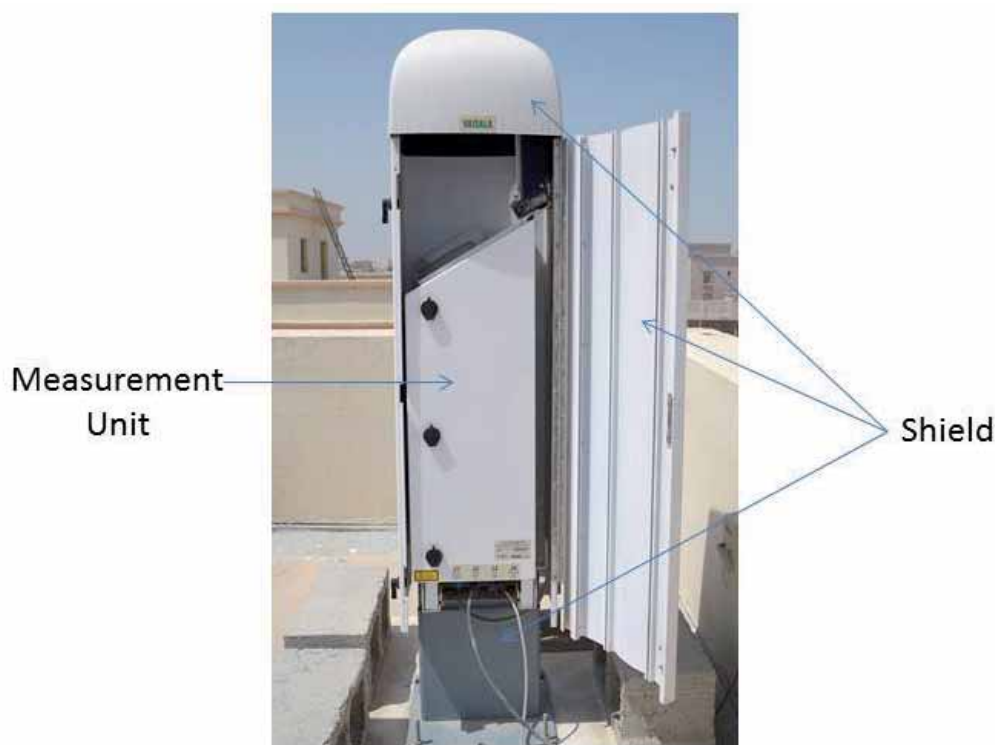
Figure 4.1: Vaisala Ceilometer CL51, as installed at the QEERI facility in Doha, Qatar.
