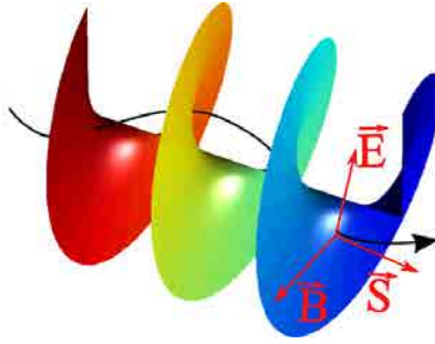
Figure 2.6: In the immediate vicinity of a vortex, the azimuthal phase term produces an optical field with a helicoidal wave front
