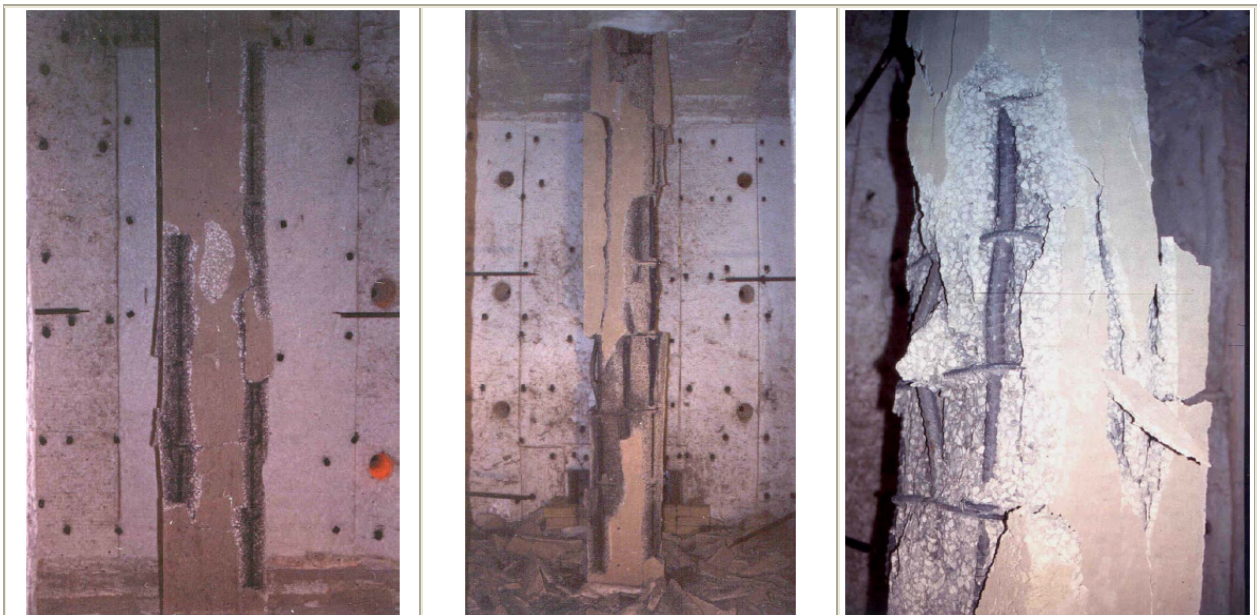
Figure 7-2. Corner Thermal Spalling examples during Fire Resistance Tests [3].
