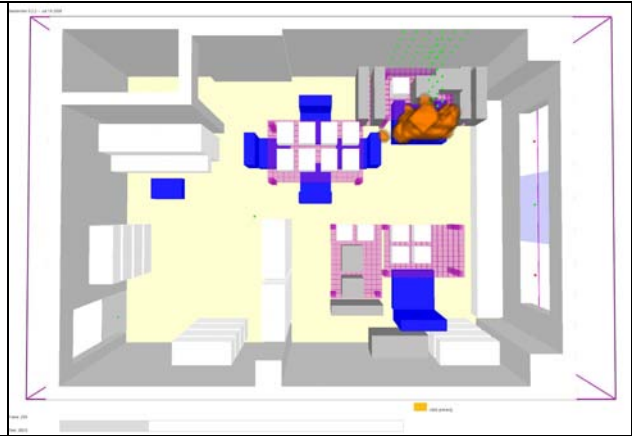
360,0 s: The west window breaks due to its temperature (300 °C).
