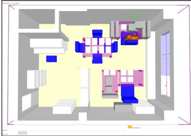
119,5 s: Fire at chair cushion after 2 minutes of ignition.
