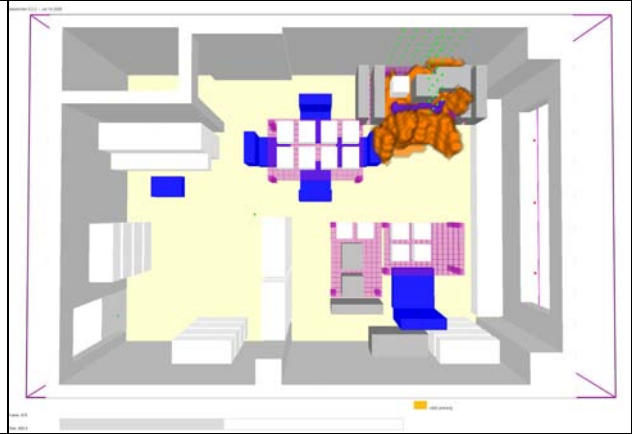
664,4 s: The middle window breaks due to its temperature.
