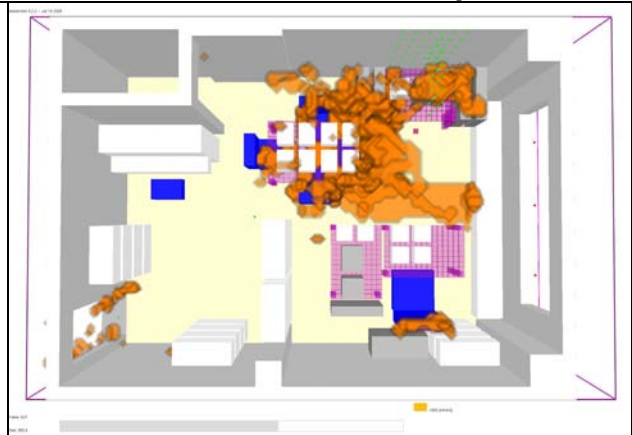
885,4 s:Flames reach the entrance door. Flashover has already happened.
