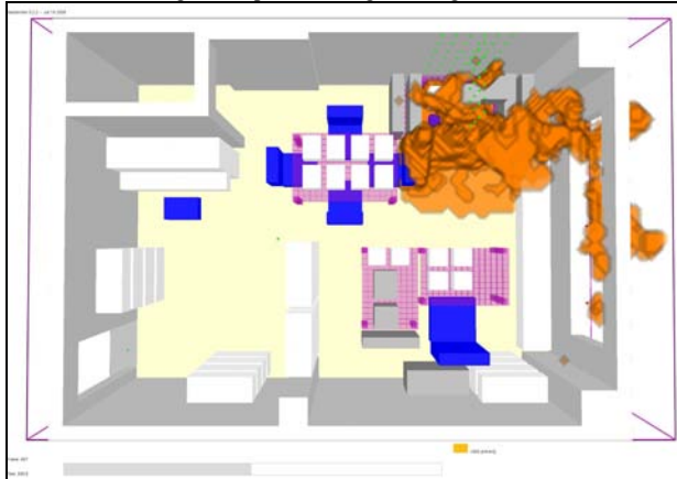
690,8 s: Big contribution of oxygen due to the middle window break.
