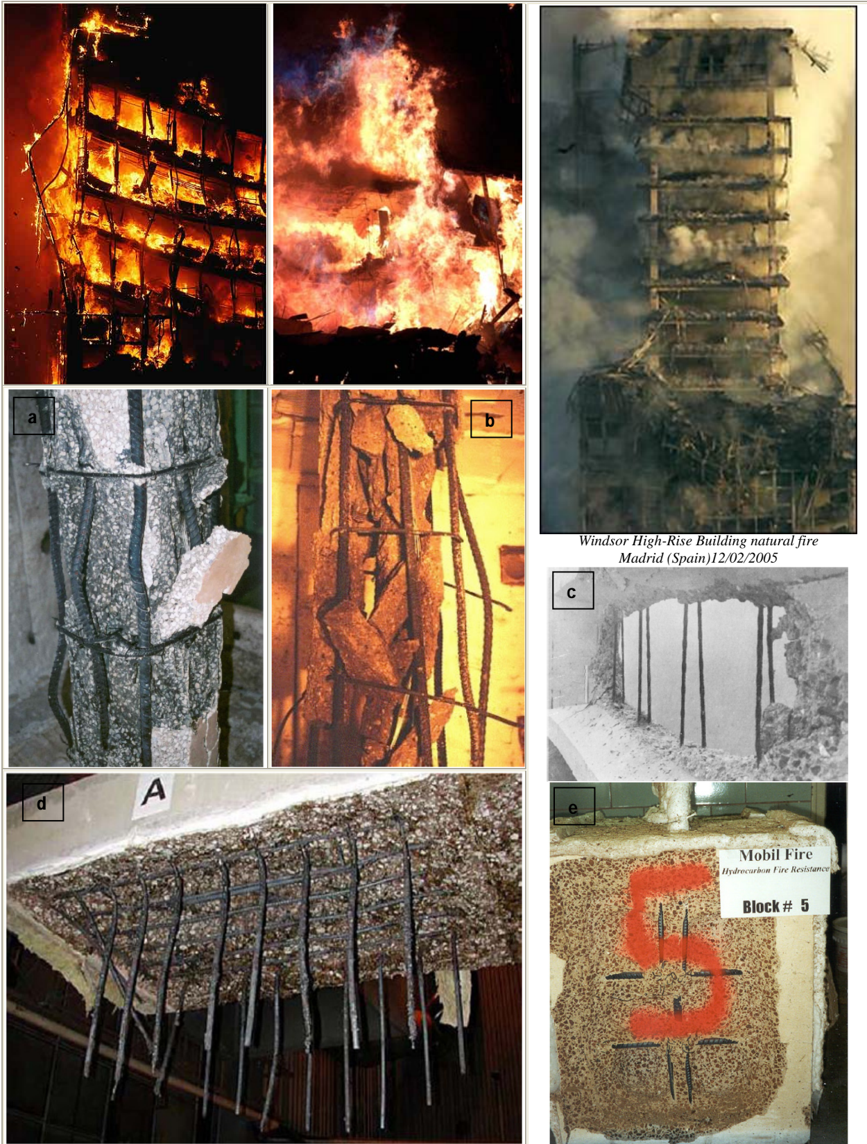
Figure 1-3. Some examples of Thermal Spalling events and their environment (I of II).
