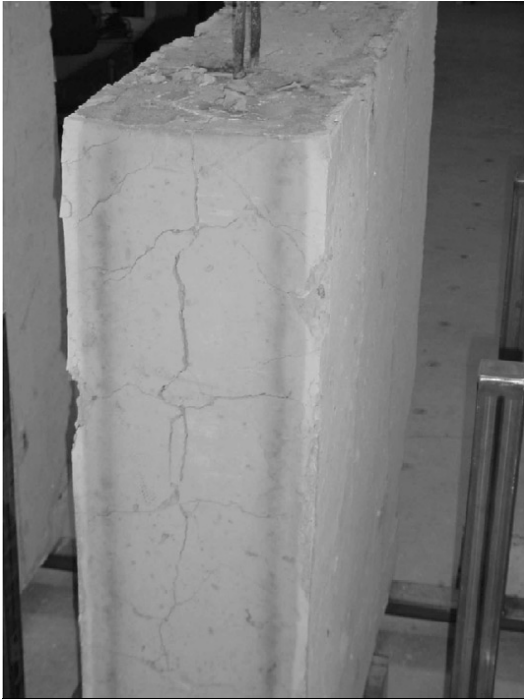
Figure 4-2. Thermal cracks in a test wall element of dense concrete (excerpt from [12]).
