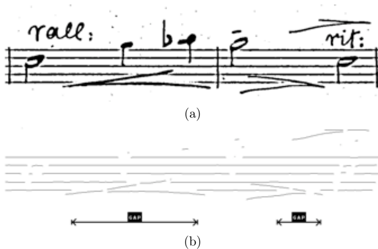
Figure 8.7: (a) Original Image (b) Line segments of staff lines with gaps and horizontal symbols.
