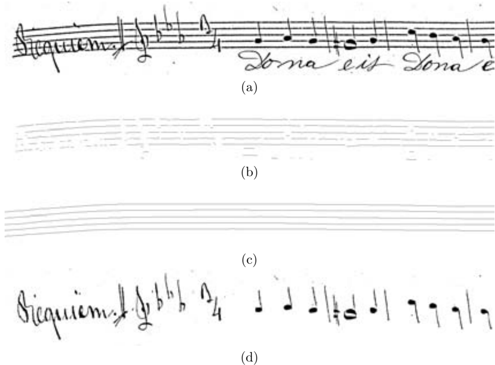
Figure 8.8: (a) Original Image; (b) Horizontal segments of the score; (c) Reconstruction of the hypothetical staff lines. (d) Image without staff lines nor lyrics.
